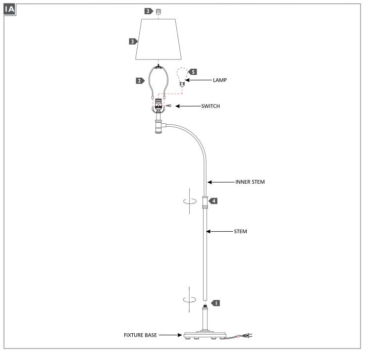
**I** Screw the stem into the fixture base.
